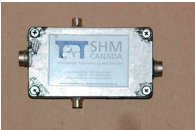
Figure 3: Left: Digital Sensor Interface (DSI). Right: Strain gauge installation
