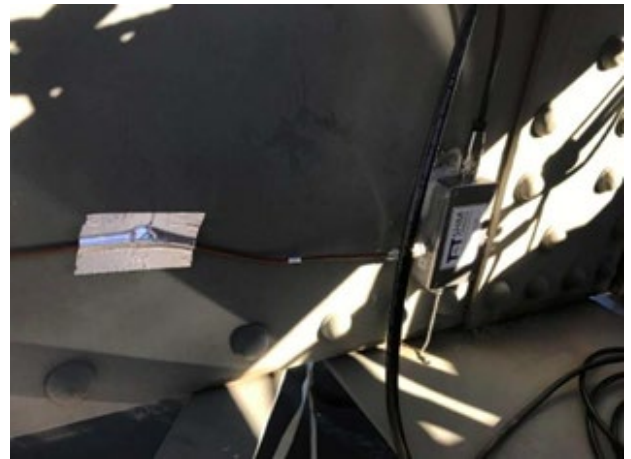
Figure 3: Left: Digital Sensor Interface (DSI). Right: Strain gauge installation
