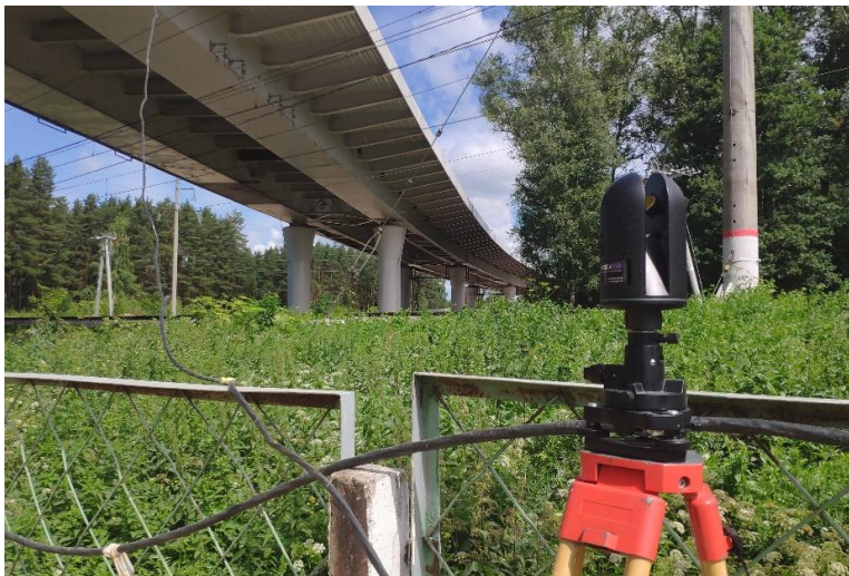
Figure 6: The process of 3D laser scanning of the overpass
