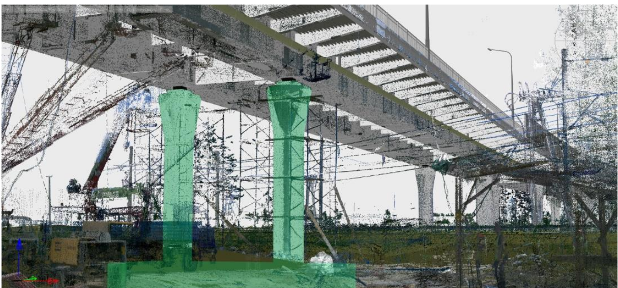
Figure 7: Visual comparison of the point cloud with the information model. Bottom view
