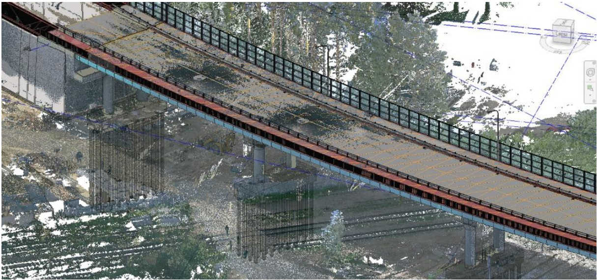
Figure 8: Visual comparison of the point cloud with the information model. Top view
