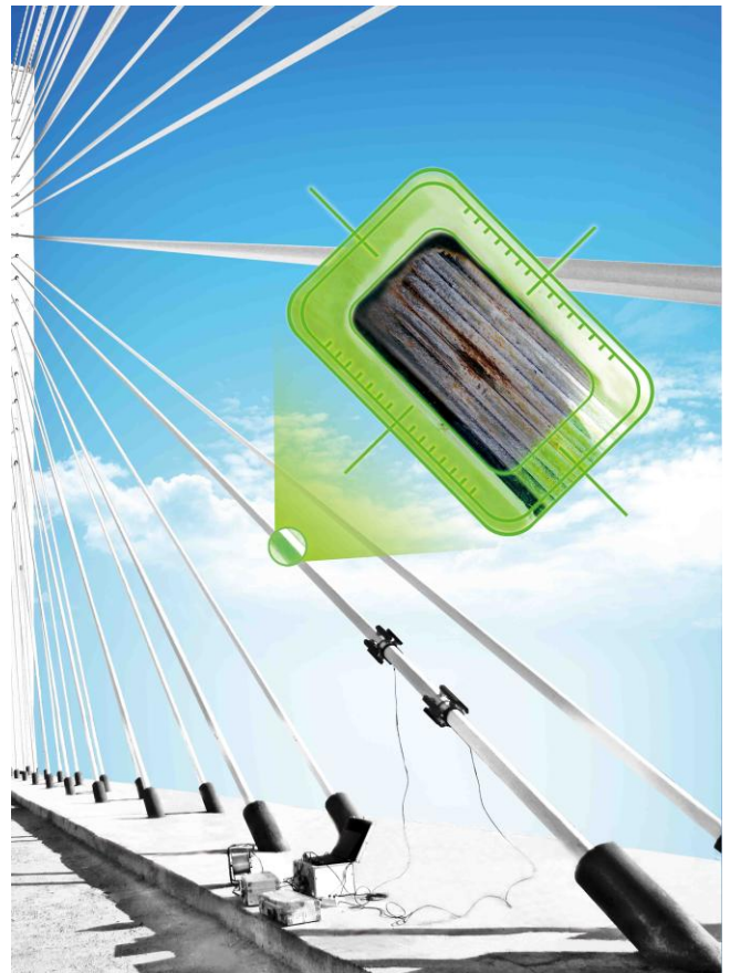
Figure 2: Detection of internal corrosion and broken wires in cables
